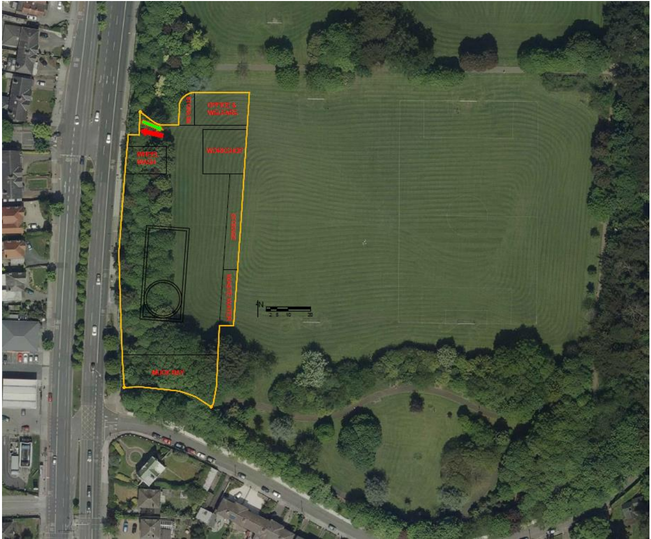
Figure 13 – Proposed Extent of Compound for Shaft Construction
