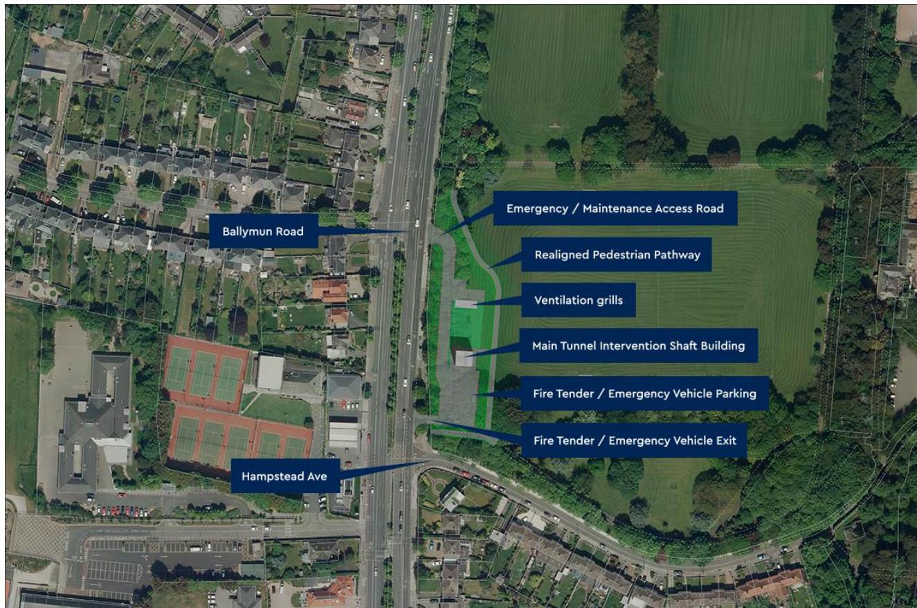
Figure 10 – Road Access and Emergency/Maintenance Vehicle Parking
